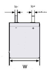
Height h:  $4.5 \pm 0.3 \text{ mm}$ Width w:  $63.5 \pm 1.5 \text{ mm}$ Length I:  $77.5 \pm 2.0 \text{ mm}$
