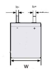
Height h: 4.2 + 0.2 mmWidth w:  $32.5 \pm 0.2 \text{ mm}$ Length I:  $48.5 \pm 0.15 \text{ mm}$
